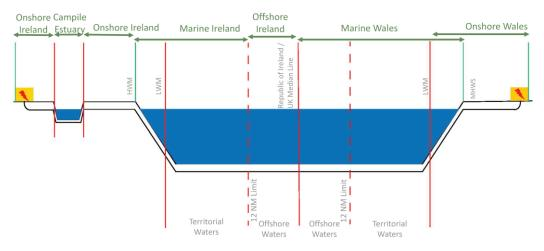
Figure 1.2 Greenlink Components | not to scale
